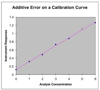
a negative instrument response, since there would be no fingerprint on the cuvette. That would be an immediate clue that there was an additive error in the standard measurements.
