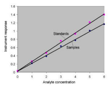
curve caused by systematic errors such as using different cuvette path lengths can be referred to as a change in sensitivity ... that is, a change in the instrument response per unit concentration. Such
