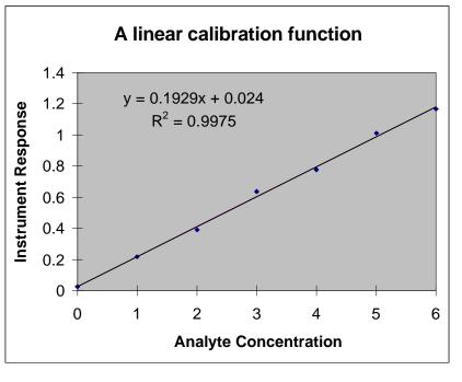
of a series of standards using a UV-vis absorption spectrophotometer, you unknowingly place a fingerprint on the absorption cell. Instead of a plot as shown above, you get a line that is offset from the origin on the y-axis by the instrument response resulting from the fingerprint. It will be the same at all analyte concentrations.
