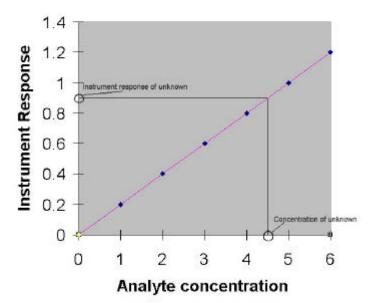
function was nonlinear, it would not be as easy to define and more sensitive to changes in physical phenomena. There would be greater error on any concentration determined from a nonlinear instrument response. So, what you want and what you most often see is a linear calibration function in analytical chemistry.
